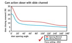
DORMA's unique cam action closer combined with a slide arm and channel do not experience an increase in the opening resistance but a rapid fall in opening resistance on operation of the door.
