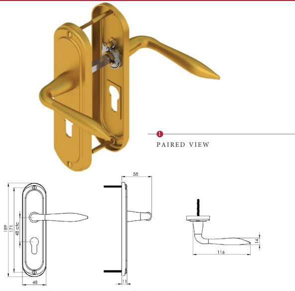
This lock handle is suitable for use with most U.K. Euro Profile cylinders and sashlocks with a  $48 \mathrm{mm}$  CTC.
