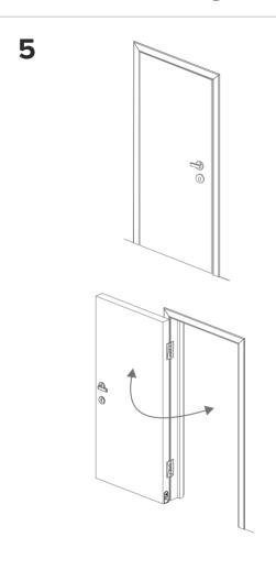
**5** Open and close door to test seal drop.
